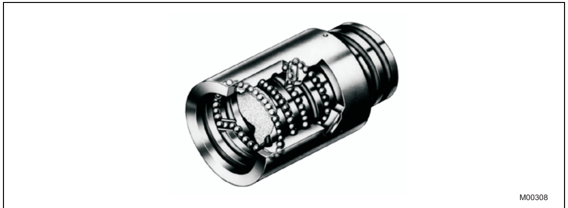
Fig. 12: Ball bearing screw with nut, cross-section
