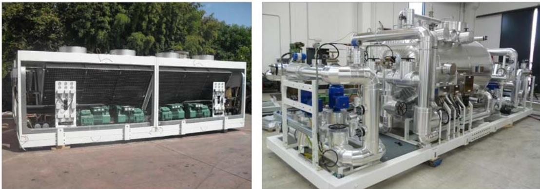
Figure 3: Chiller system: refrigerant unit and water tank skid
