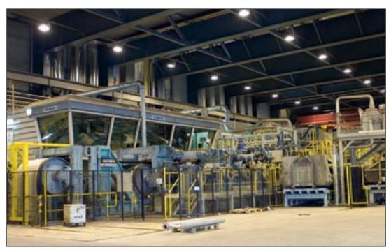
The continuous RAP 5 line consists of a three-stand tandem mill, annealing and pickling units, a skin pass mill and a tension leveling unit. The line is 800 m long and occupies all of the three floors of the No. 2 cold rolling plant. The horizontal loopers allow the RAP line to be used continuously and when fully loaded, there is up to 4000 m of strip in the line.
