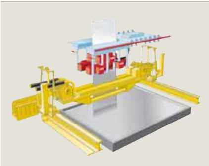
4 The stabilizer suspended from an overhead construction
