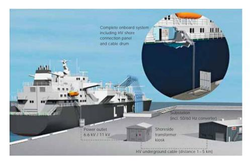
that of the vessel. As the development of an onshore power supply can have a significant impact on the local grid, ABB also offers system studies to assess the overall effect, and can recommend solutions to upgrade and strengthen the local grid and port network to accommodate shore power connections.
