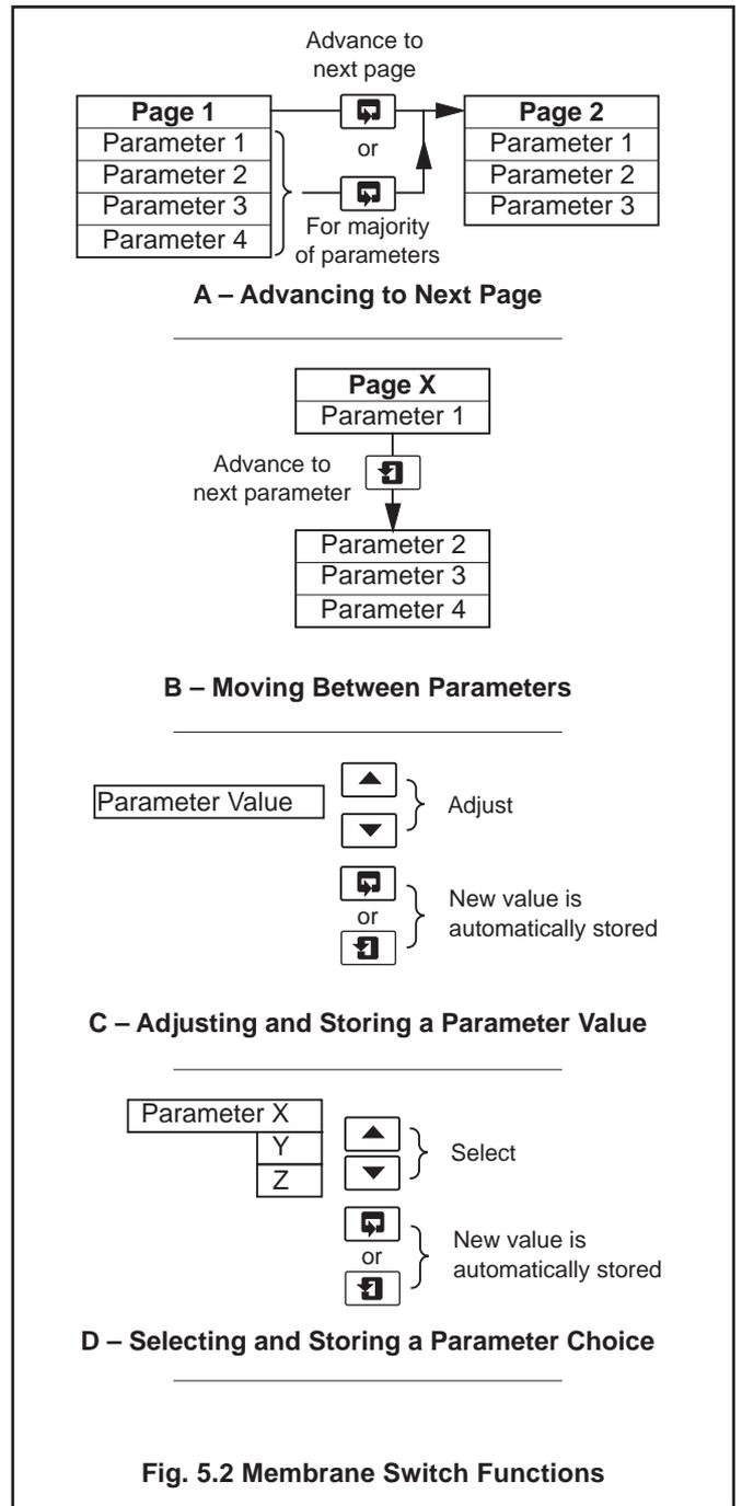
Fig. 5.2 Membrane Switch Functions
