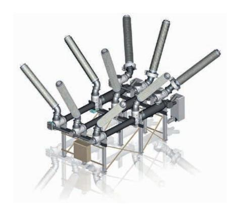
To make transportation of the fully assembled product possible, the insulators are rotated in the factory from the in-service position to the transport position, and back again at the installation site.
