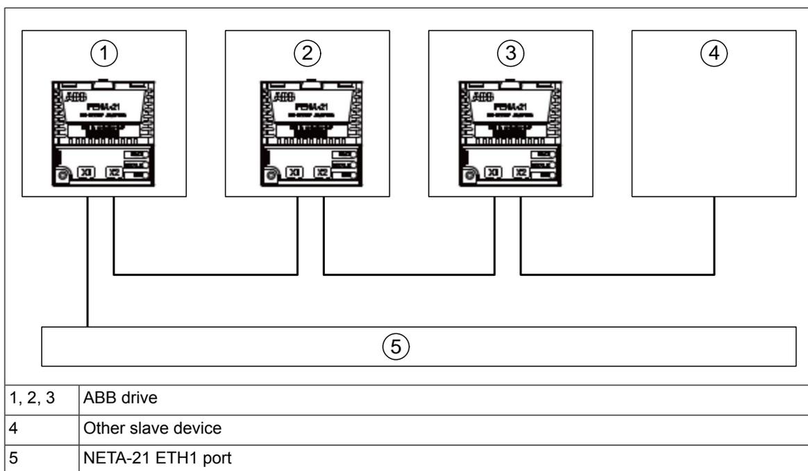
One of the Ethernet port of a NETA-21 must be connected to internet (cellular modem) and the other Ethernet port can be connected for local monitoring (FENA-21 adapters in drives). The gateway is configured only for the Ethernet link which is connected to the internet.
