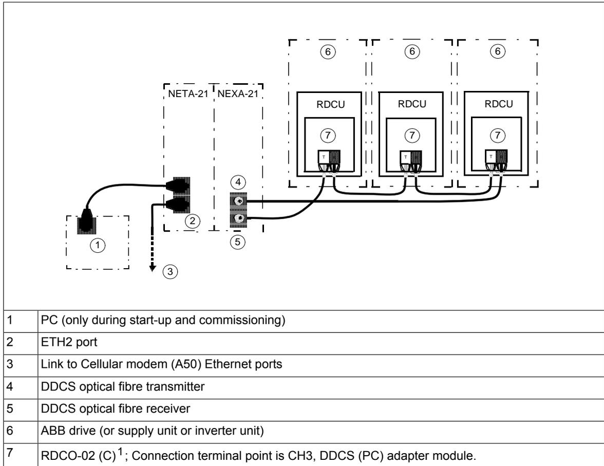
Connect the NEXA-21 primarily to fiber optic channel CH3 on the RDCO-02 (C) module.
