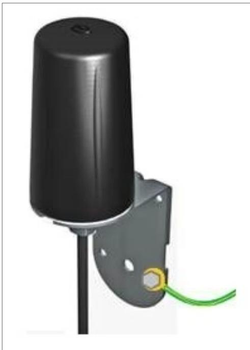
5. Ground the antenna mounting bracket with 6 mm<sup>2</sup> earthing conductor.
