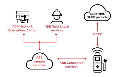
Connected Services ABB E-mobility connectivity solutions link EV chargers to back-end systems as well as robust service tools.
