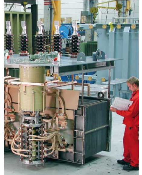
Series reactor with on-load tap changers, OLTC
