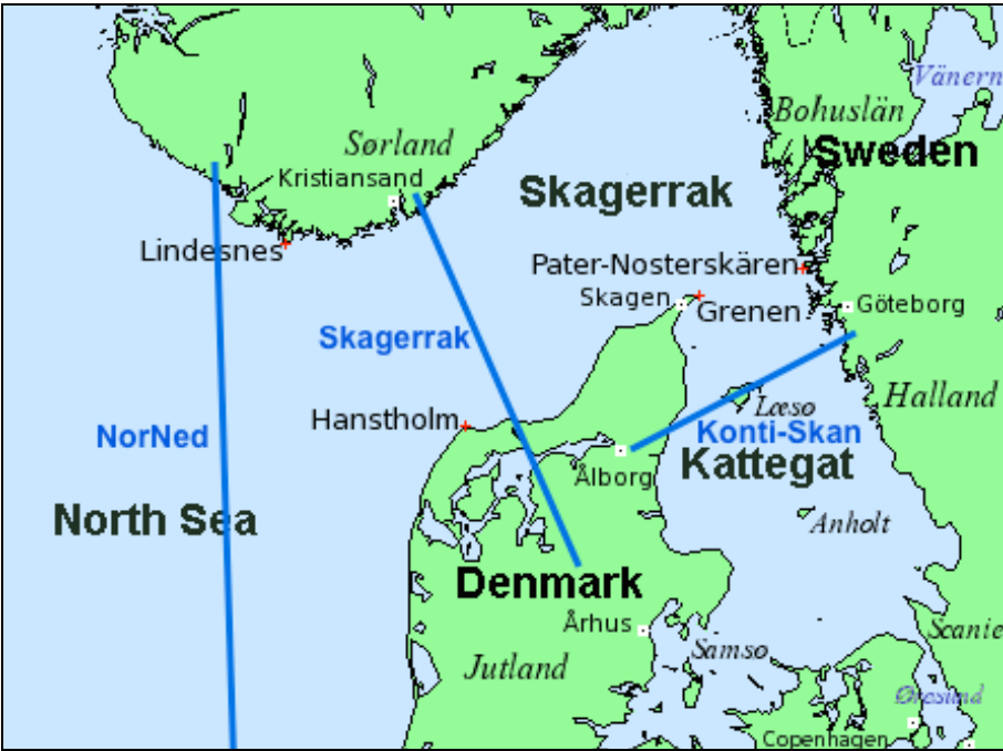
Figure 1. Skagerrak, Kont-Skan and NorNed HVDC links
