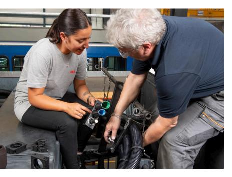
The flexible PMA TRUST™ modular support system offers many options for securing cables and conduits. The new solution also benefit Bernmobil in Bern, Switzerland: The city's public transport operator, carries over 100 million passengers annually on its network of 5 tram routes, 3 trolley bus routes and 26 bus routes.
