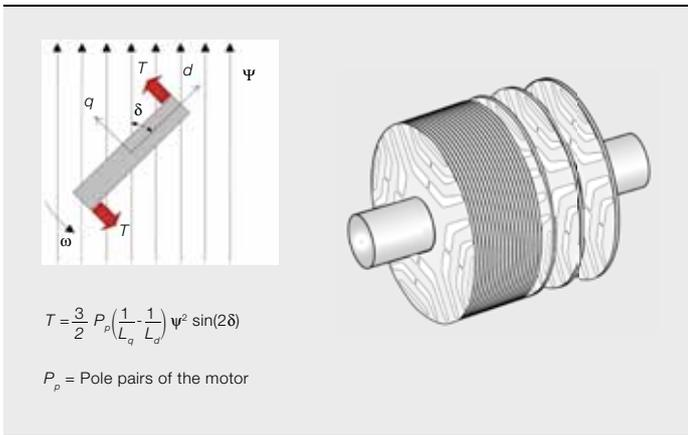
magnetically conducting direction to the stator field. The strength of the produced torque is directly related to the saliency ratio, ie the inductance ratio between the two magnetic directions of the rotor.
