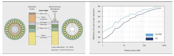
studies bearing failure is the root cause of approximately 70 percent of all unplanned motor outages. The lower bearing temperature directly translates into longer greasing intervals, reduced maintenance and higher reliability. Even if a bearing eventually needs replacing, having no magnetic forces, unlike a PM motor, the bearing change is as easy as for an IM.
