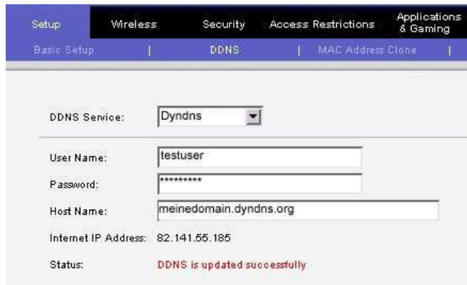
Figure 150: DynDNS Router settings
