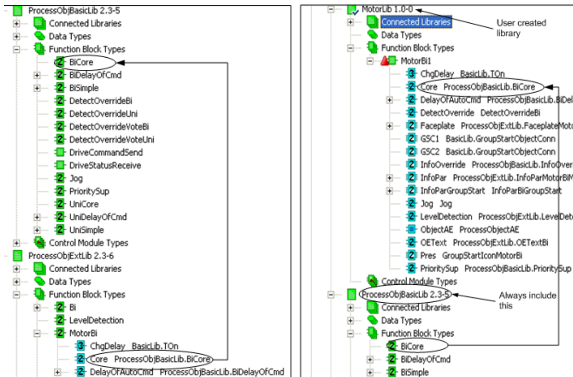
Figure 121. The core functionality in ProcessObjExtLib and in a user's self-defined library
