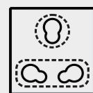
Socket with separate shutter
