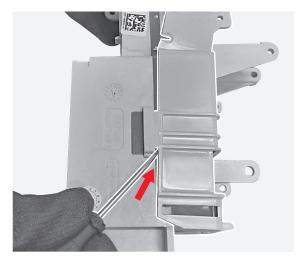
By means of the flat screwdriver unhook as indicated by the arrow the flat cover from the MID main structure.
