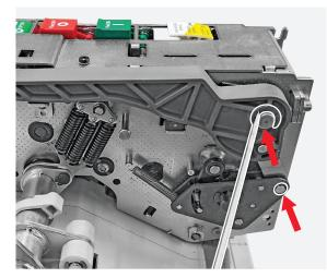
**179** By means of the flat screwdriver remove the benzing.
