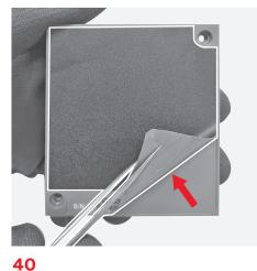
Manually remove the Ekip measuring blind case.
