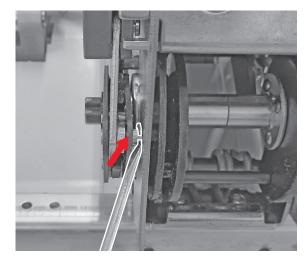
Manually remove the pin and the nut.
