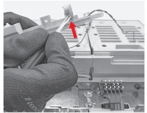
By means of the flat screwdriver remove the clip and after manually complete the removal.
