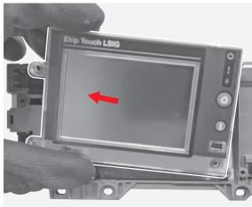
By means of the cutter start removing the trip unit front label and by means of the pliers complete the operation.
