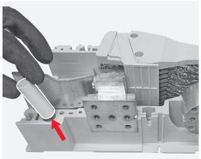
Manually remove the insulating protection.
