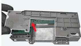
By means of the flat screwdriver unhook the trip unit printed circuit board.
