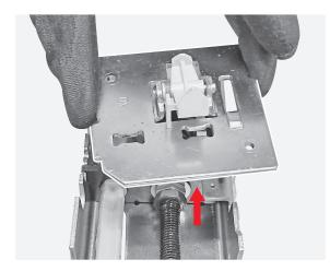
By means of flat screwdriver remove the benzing.
