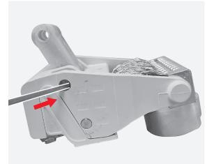
Manually remove the pin and the tie rod.
