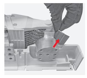
**244** Manually remove the mobile contact. 243
