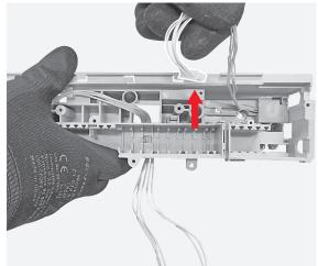
By means of the flat screwdriver unhook the 2 microswitches from their support and after separate the microswitches support from the rest of the connector.
