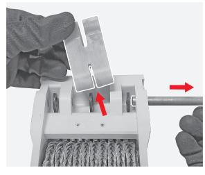
**250** Manually remove the insulation protection.
