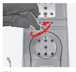
**234** By means of the flat screwdriver unhook the sensor plug mounted below the sensor and after manually remove the sensor plug.
