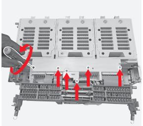
Manually remove the base and the cover.
