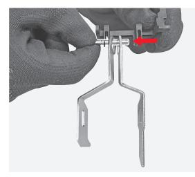
**137** Let fall by gravity the mechanical reset anchor.
