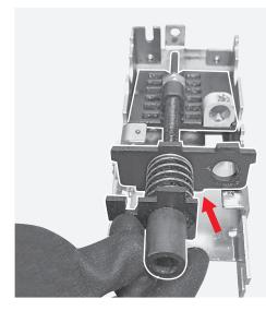
By means of the flat screwdriver remove the benzing and after manually remove the feeler.
