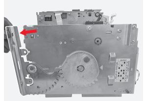
Manually remove the assembly shaft.
