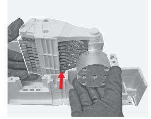
**246** Manually remove the jumper.
