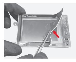
**62** Manually remove the battery.
