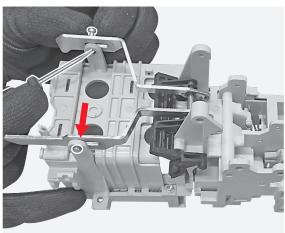
Manually remove the assembly mounted on the MID main structure.
