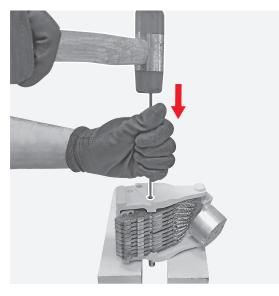
**253** Manually separate the mobile contact from its contacts holder.
