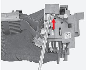
By means of the flat screwdriver unhook the right side wall from the sliding contacts main assembly as indicated in the picture.
