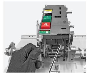
By means of the flat screwdriver push as indicated by the arrow the pin and remove the pin.
