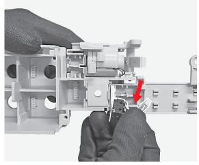
By means of the flat screwdriver slightly lift up the appendix as indicated by the arrow and manually remove the trip coil assembly.
