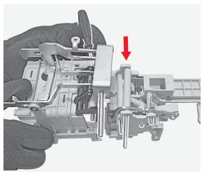
**132** By means of the flat screwdriver remove the 2 pins.
