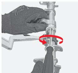
Manually remove the cam.
