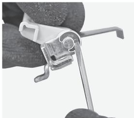
By means of the flat screwdriver push the pin as indicated by the arrow and let the the I/O shaft, the I/O shaft group support and the leaf spring constituting the I/O shaft group separate.
