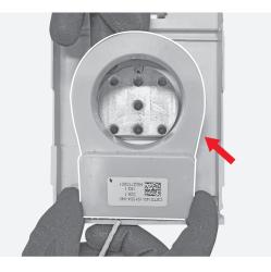
Manually unhook the cable from the sensor.
