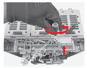
Push the flat srewdriver in the direction indicated by the arrow and after manually remove the microswitch assembly.
