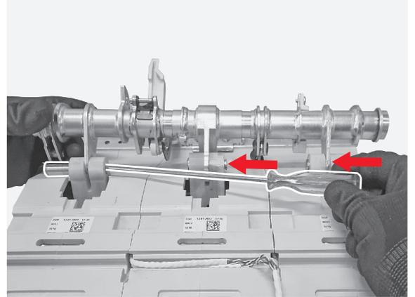
**191** Manually remove the operating shaft assembly.
