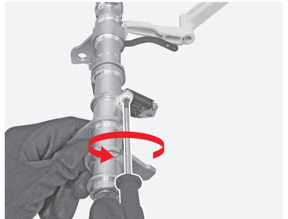
**193** Manually remove the auxiliary contacts cam.
