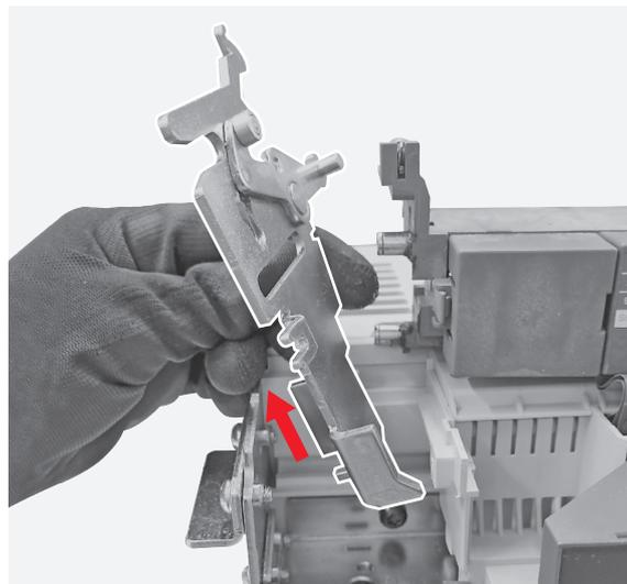
**22** Move the sliding contacts block as shown in the picture and by means of the torx key unscrew the 6 screws fixing the base and the cover.
