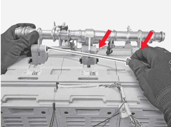
**190** Manually lift the operating shaft assembly and by means of the flat screwdriver remove the 3 pins.
