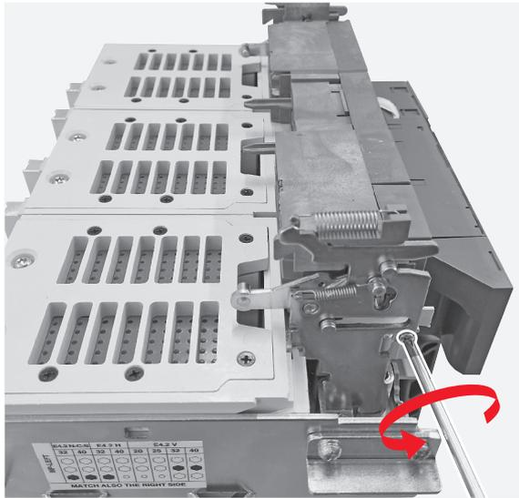
**20** By means of the cross screwdriver unscrew the 1 + 1 screws fixing the 2 sides walls located at both sides of the sliding contacts block to the circuit breaker main structure.
