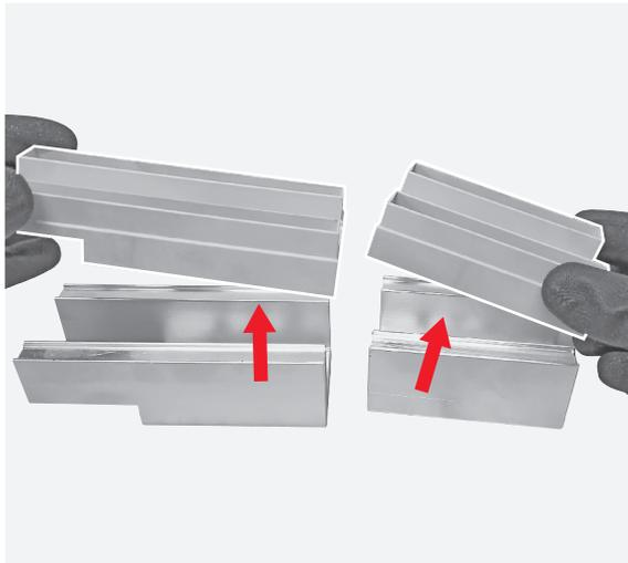
Disassembly operations illustrated at pictures 204, 205 and 206 must be performed on the other 2 poles.
