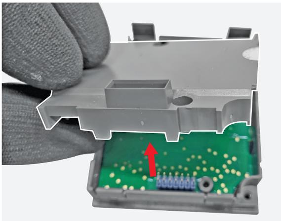
**41** Manually remove the printed circuit board.
