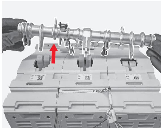
**192** By means of the cross screwdriver unscrew the screw fixing the auxiliary contacts cam to the operating shaft assembly.
