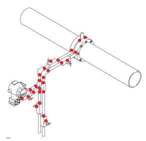
Traditional orifice installation highlighting potential leakage points
