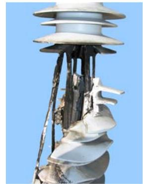
Figure 4. Failed short circuit test during trial without belt-winding.
