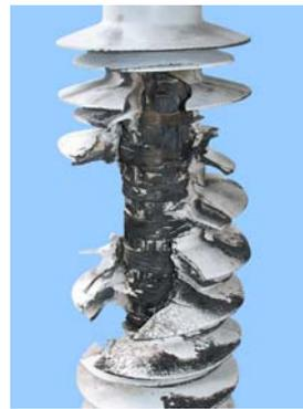
Figure 3. Successful short circuit test on PEXLIM surge arrester with belt-winding.
