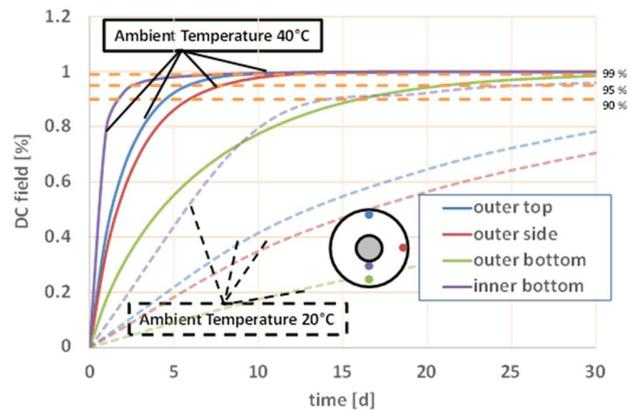
Figure 8 Transition time for the insulator, depending on the location and ambient temperature
