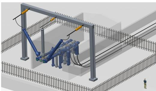
Figure 10 Gas-insulated cable to overhead line transition station
