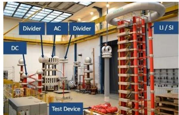
Figure 4 Test arrangement for superimposed voltage tests
