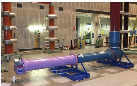
Figure 2 type test of the RC-divider
