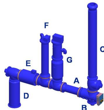
Figure 1 HVDC GIS components
