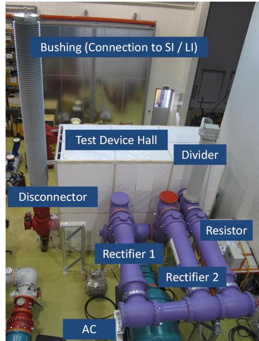
Figure 6 DC insulation system: test set-up
