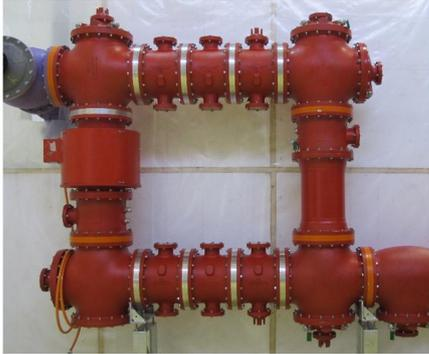
Figure 7 DC insulation system test: test device (partitions)
