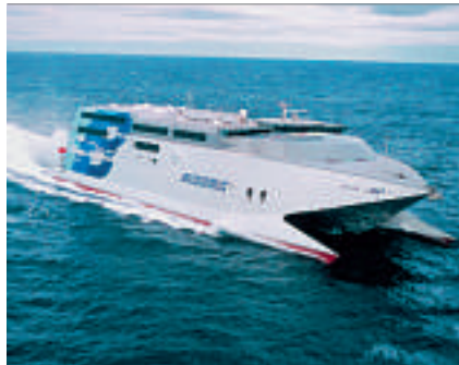
6 Buquebus Line's fast ferry Catalonia, with eight TPL65A turbochargers on its four caterpillar 3618 engines, broke the record for the quickest surface transatlantic crossing in 1998.
