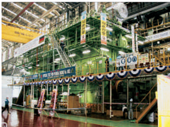
9 Testing at Hyundai Heavy Industries in Korea of the world's most powerful electronically controlled 12K98ME MANB&W engine, with three TPL91-B units, under full load (93,360 bhp).
