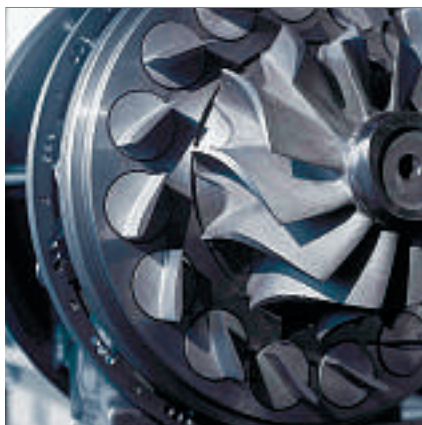
4 Variable nozzle ring of a TPS57 VTG turbocharger.
