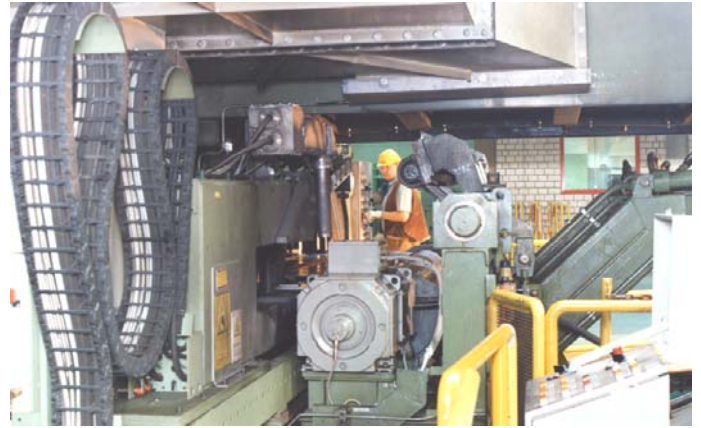
Fig. 3 Exit side with drive for flatness measurement roll, laser and X-ray strip thickness gauge
