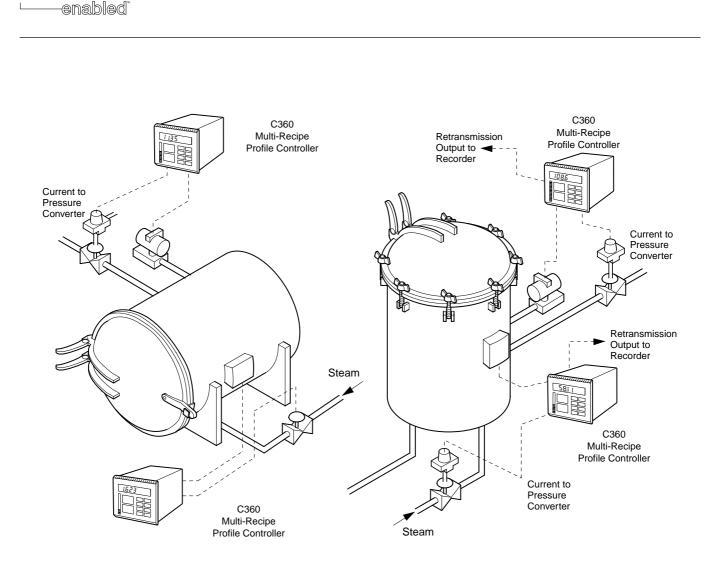
Fig. 1 Horizontal and Vertical Retorts
