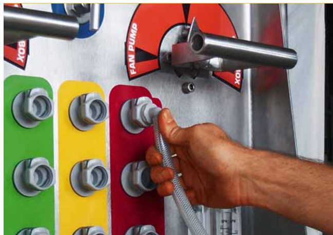
3 Well labeled, or color coded valves and connections are intuitive. They speed setup, and reduce mistakes.
