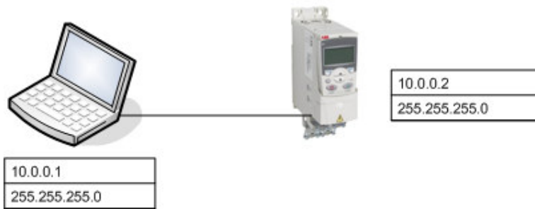
Figure 1. Point to point connection with a crossover cable.
