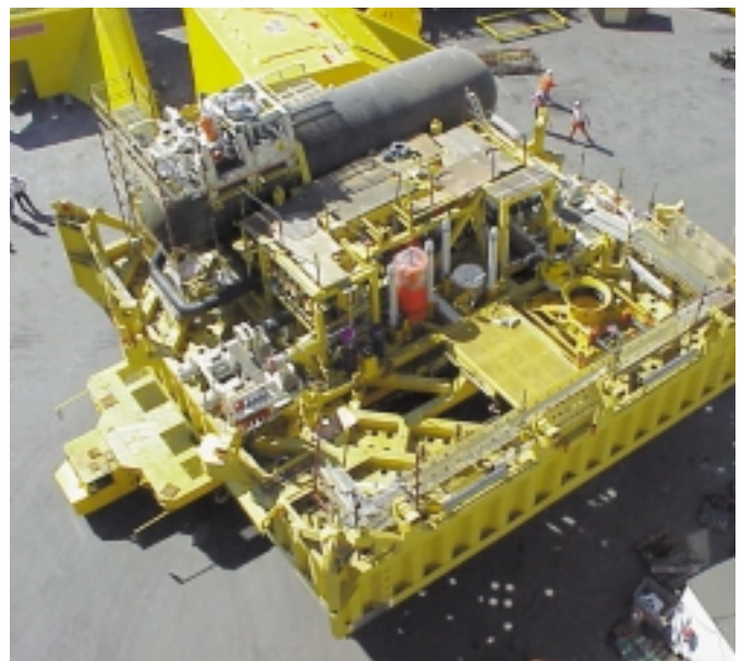
9 SUBSIS™, the world's first subsea separation and injection system, being prepared for the Troll Pilot project in the North Sea
