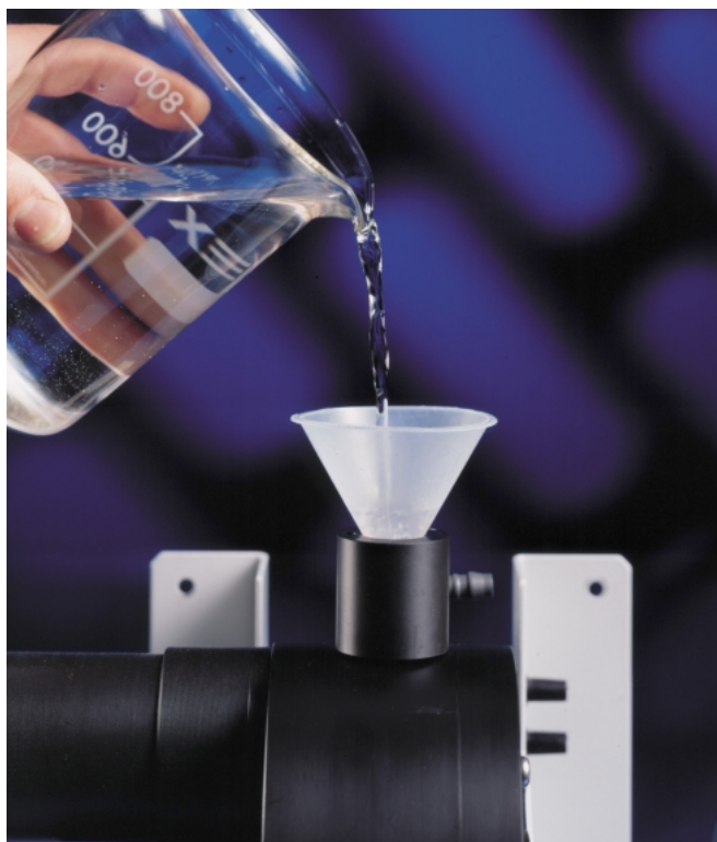
Adding Demineralized Water for Calibration
