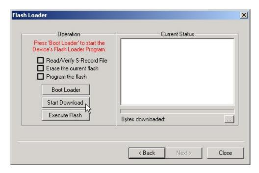
G) On the XFC display, "Totalflow Flash Loader" will appear on the top line and Erase" on the bottom line. Next, on the display "Flash Loader" will start to increment numbers until it is complete. The "Flash Loader" screen will appear as below during the Flash Download.
