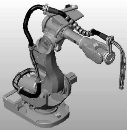
Figure 66 "Orange line" DressPack Upper/Lower arm SpotWelding (option 778-2, option 781-1 and option 798-2).
