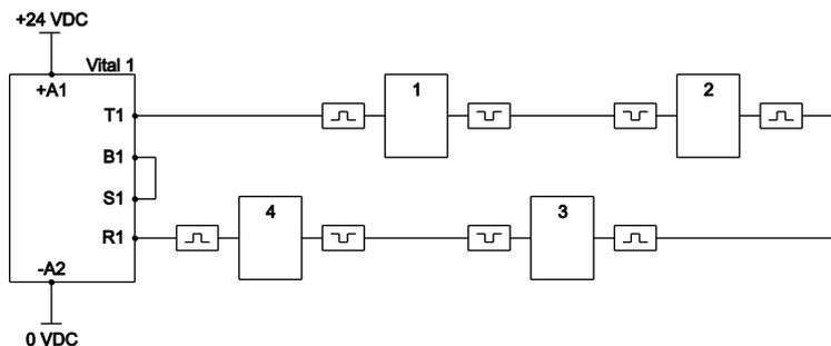
Vital 1 with an even number of sensors connected in series between T1 and R1. S1 connected to B1.
