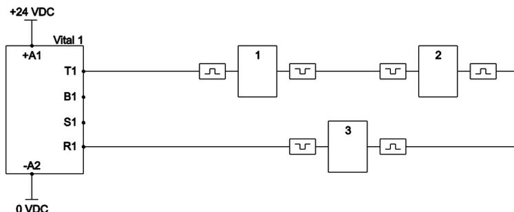
Vital 1 with an odd number of sensors connected in series between T1 and R1. S1 disconnected.
