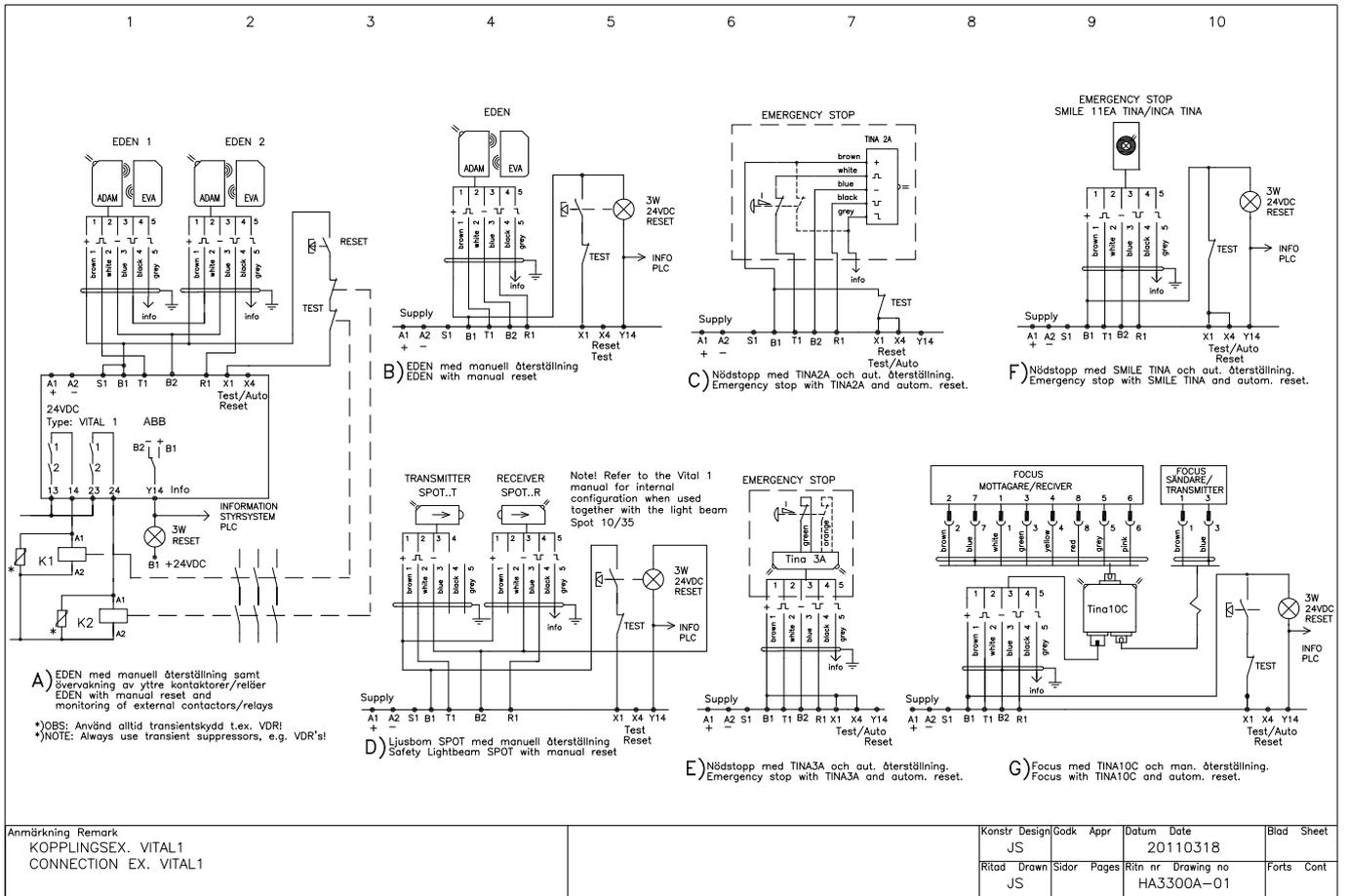
**NB:** If the safety light beam Spot 110/35 is connected to Vital 1, the information output switch must be in position 2. See section *Output connections* for further details.
