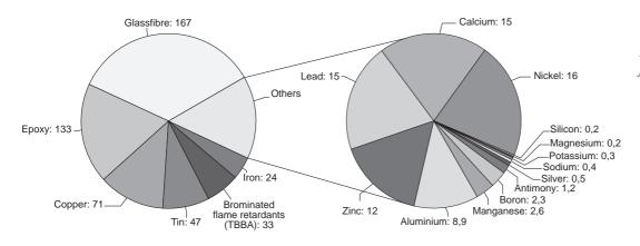
Figure 4. Material content for circuit boards<sup>2</sup>.
