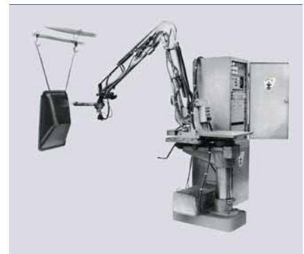
3 Early version of the Trallfa paint robot from 1969
