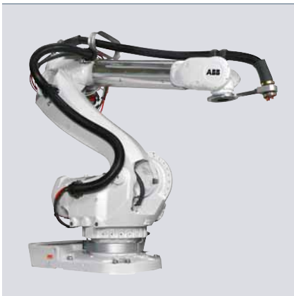
5 The IRB 6000 with its modular design concept was introduced in 1991 and became ABB's best-selling spot-welding robot.
