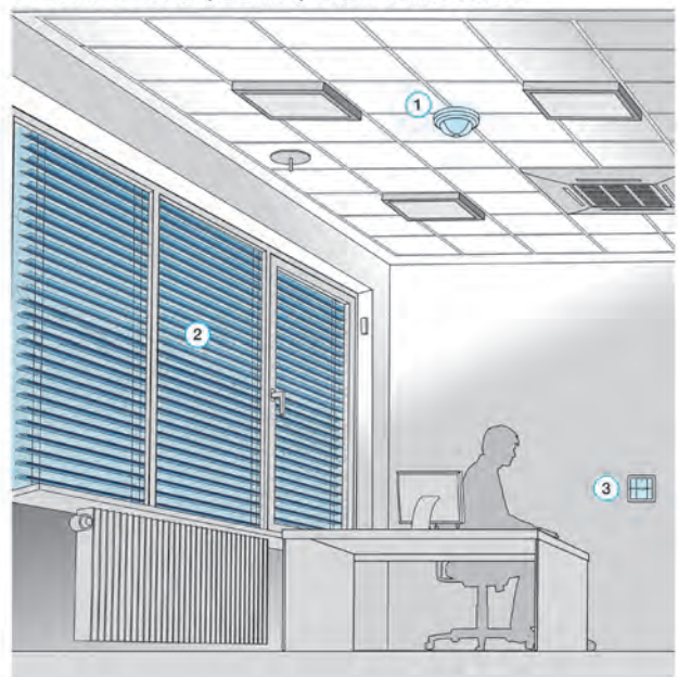
1 Presence detector | 2 Blind | 3 Manual blind control
