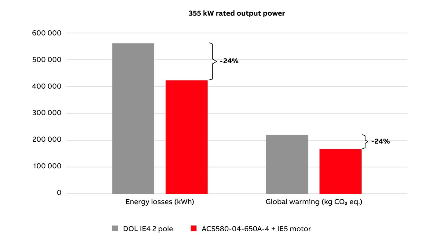
Use stage energy losses and contribution to global warming of ACS580-04-650A-4 VSD + IE5 VSD motor system and an equivalent DOL motor.
