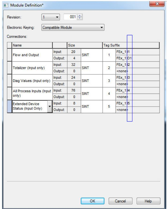
To see the cycle-time-configuration as **Requested Packet Interval (RPI)** in milliseconds, navigate to the **Connection** tab.
