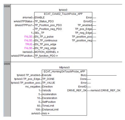
IMPORTANT: The touchprobe and homing blocks should always be in a program element called by the EtherCAT related task
