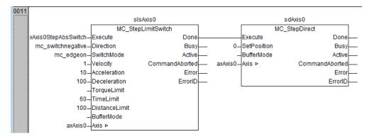
The example is hard coded to run the axis in the negative direction (the Direction input of the function block is set to mc\_switchnegative) and so the home completes when the negative limit switch is activated.
