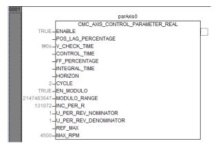
Our project was designed around a MicroFlex e190 demokit that uses a servo motor with a Smartabs encoder with 131072 counts per revolution. By setting the two U\_PER\_REV parameters to 1 this scales the axis into motor revolutions.
