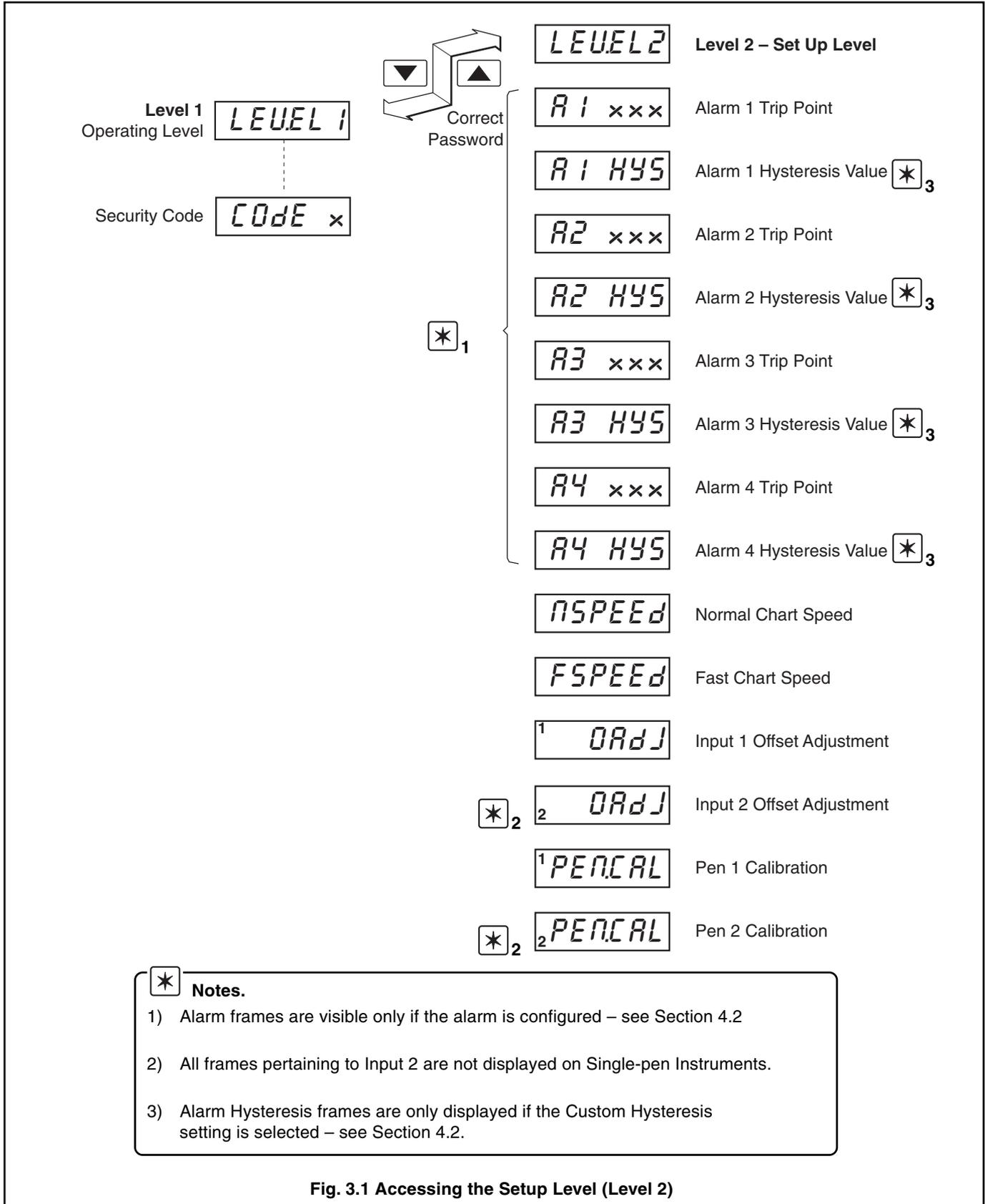
Fig. 3.1 Accessing the Setup Level (Level 2)
