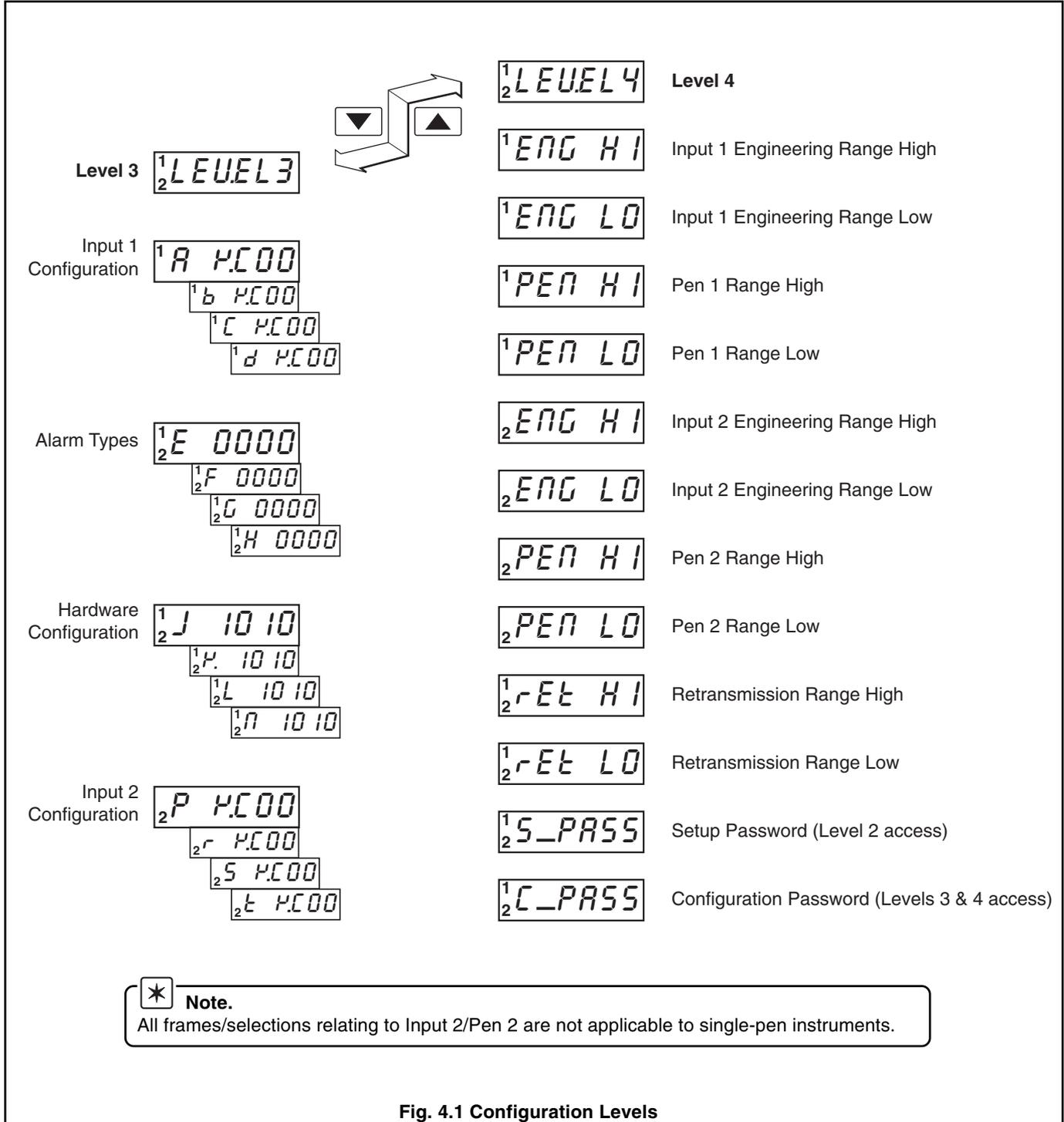
Fig. 4.1 Configuration Levels
