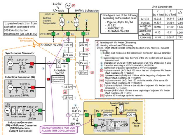
Figure 4. Study network used in PSCAD simulations
