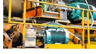
An ABB industrial drive provides a good torque response, which is vital to the control of the load in hostile crane environments, such as steelworks.
