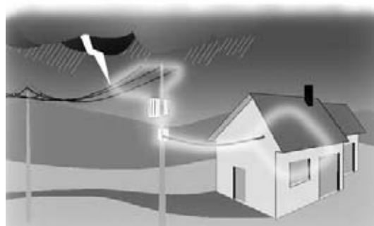
Direct lightning strike on an overhead line
