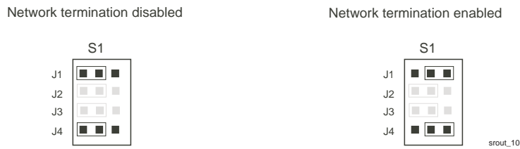
Fig. 5.2.1.-2 Jumper group S1 showing the selection of the TP/XF-78 transceiver, with network termination disabled and enabled.
