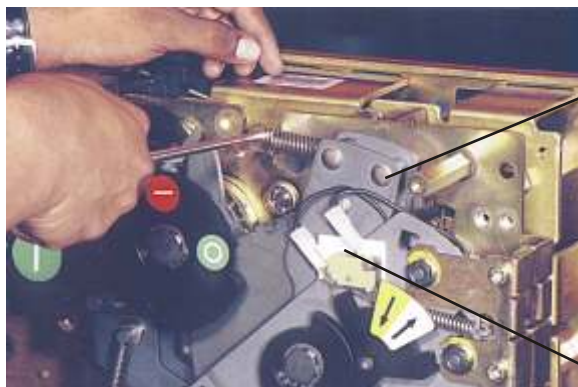
Remove the two motor limit microswitch fixing screws (2)
