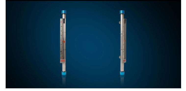
The new LMG100 Econolev magnetic liquid level gauge is designed – to address the needs of the small storage tank and OEM market. The \_ LMG100 provides armored local level indication in a simple, lower \_ cost magnetic gauge design. It is rated to 275 PSI at 200°F and has 1" FNPT side process connections.
