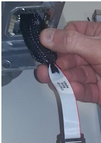
7. Connect the smart cable to the ribbon cable coming from the stamp card. Make sure the connector is securely seated.
