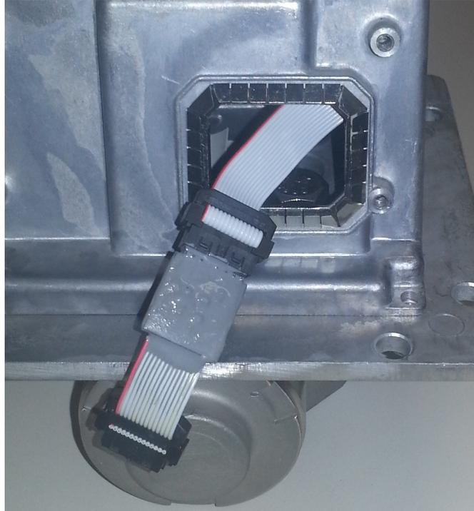
8. Ensure that the connector is fully seated and that the EMI gasket is aligned and attached properly so it will not cause shorts on the circuit board when repositioned and attached.
