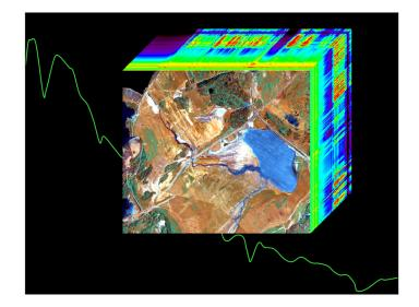
HySIS (HyperSpectral Instrument Simulator) is a collection of software models that simulate the whole processing chain of a defined hyperspectral sensor, from acquisition of spectral radiance to end data products.
