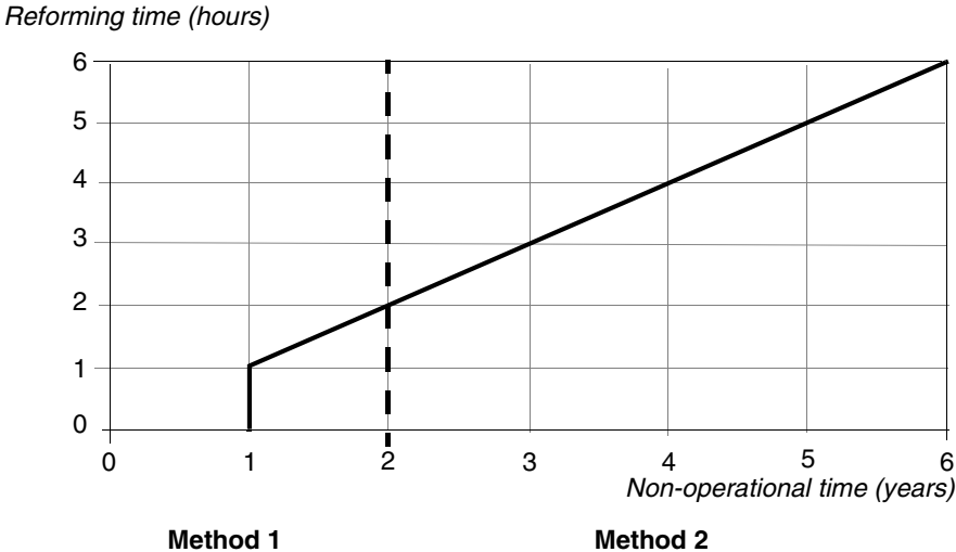
Figure 5-1 Capacitor reforming time for Method 1 and Method 2.
