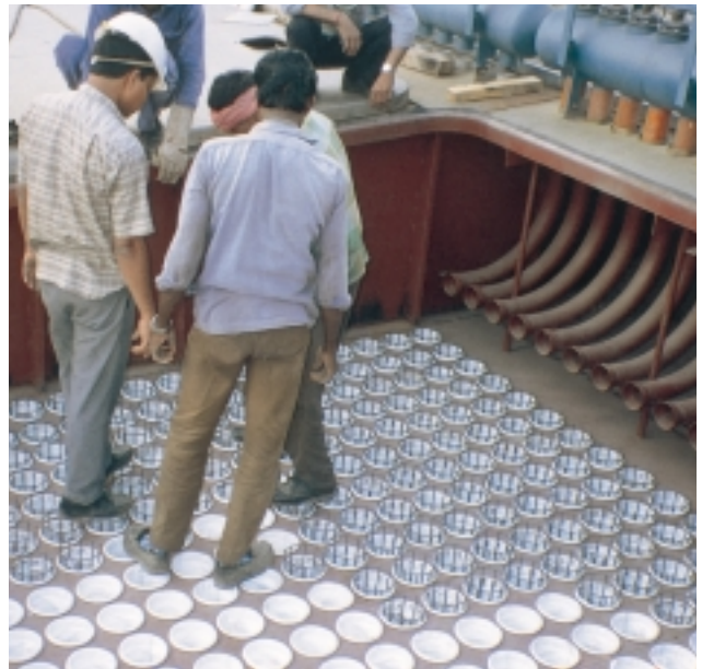
Top of a bag filter. Dense packing of the filter bags has led to a compact construction.
