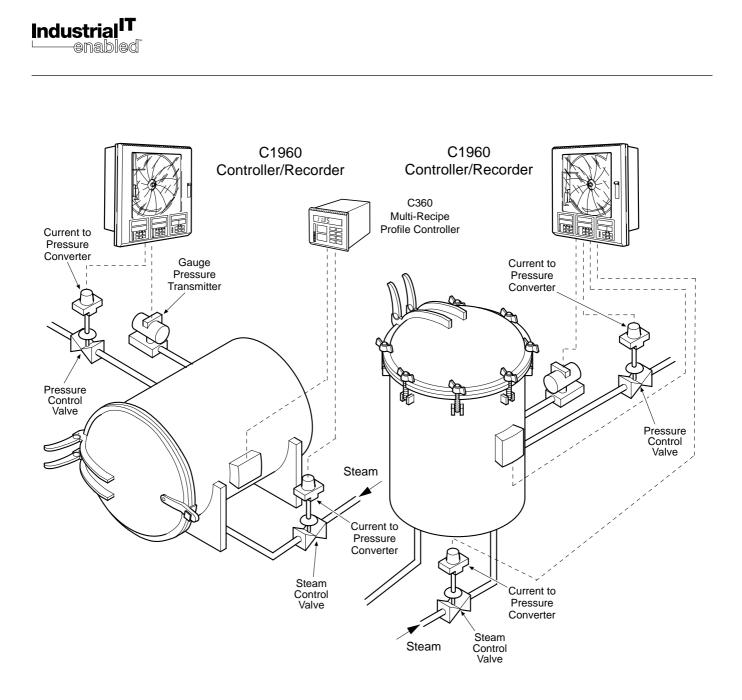
Fig. 1 Horizontal and Vertical Retorts
